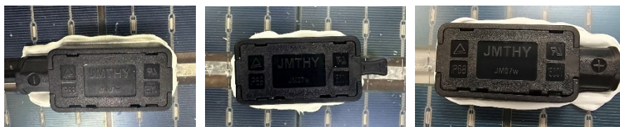
Fig. 3: View of junction box of module type ESPHSC550
